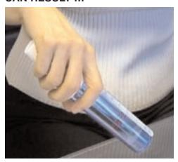
Occasionally, the resetting weight is not easily dislodged. In such cases, bang the rounded end of the meter against a hard surface (such as a table-top, although not if it is made of glass). The In-Check body was designed to withstand such attempts to dislodge the resetting weight.
